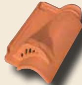
171F01 Aerator tile It is useful to keep the roof ventilated. You need one aerator tile every 25 m 2 of roof.
