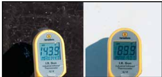
Figure 1: Dark vs. Cool Roof Surface Temperatures
